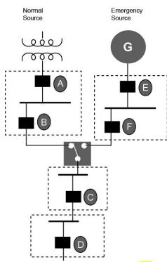
Informational Note Figure 708.54(C) Critical Operations Power System Selective Coordination. OCPD D selectively coordinates with OCPDs C, F, E, B, and A. OCPD C selectively coordinates with OCPDs F, E, B, and A. OCPD F selectively coordinates with OCPD E. OCPD B is not required to selectively coordinate with OCPD A because OCPD B is not a critical operations power system OCPD.
